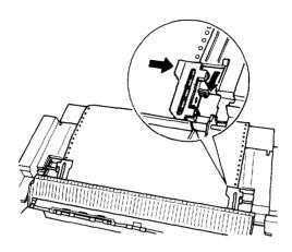
Note: Make sure the first sheet of paper has a clean, straight edge so that the paper can feed smoothly into the printer.
